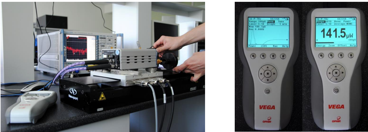
Fig. 11. Direct measurement by Ophir VEGA [10]
