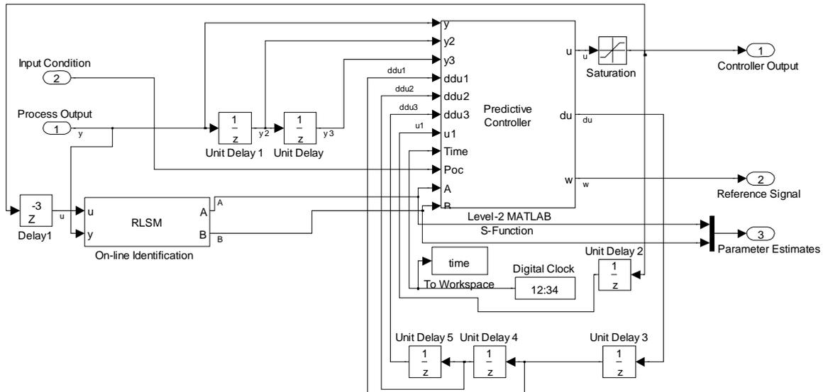
Fig. 9. SIMULINK scheme of subsystem Predictive Controller
