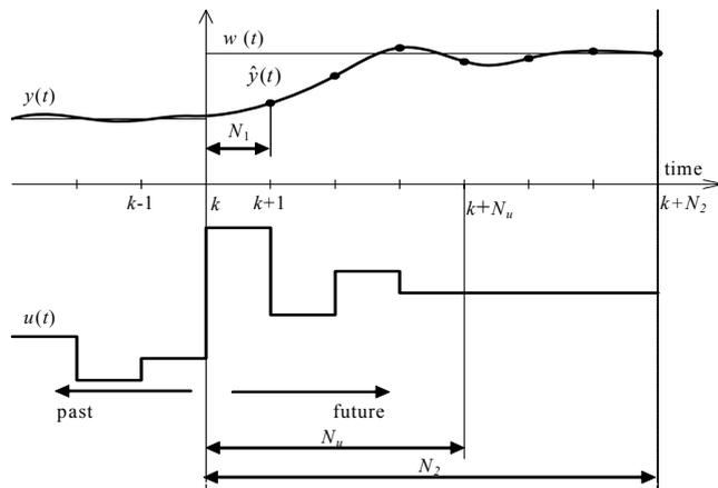
Fig. 3. Principle of MPC
