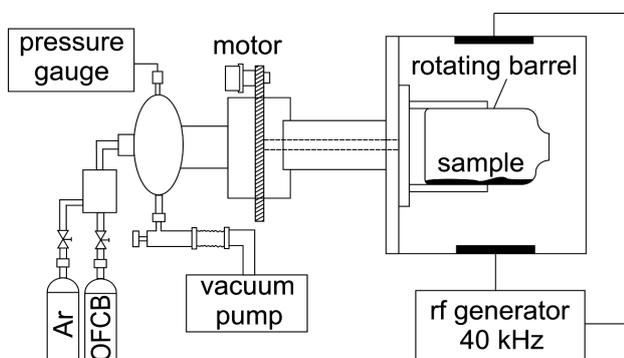
**Figure 1:** Rotary plasma reactor used for the treatment of CI particles
