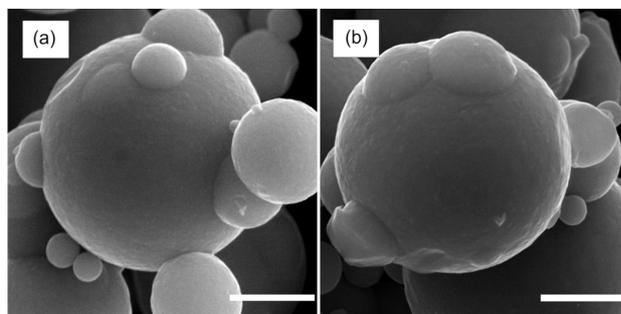
**Figure 2:** SEM images of mere CI particles (a) and plasma-treated (600 s, 100 W) CI particles (b); bar length 2  $\mu\text{m}$
