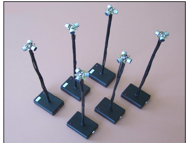
Fig. 9. Completed microphone units.
